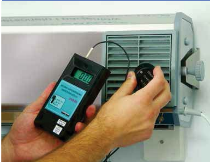
Safe to people – measurement of the irradiation with the use of counter indicates 0
